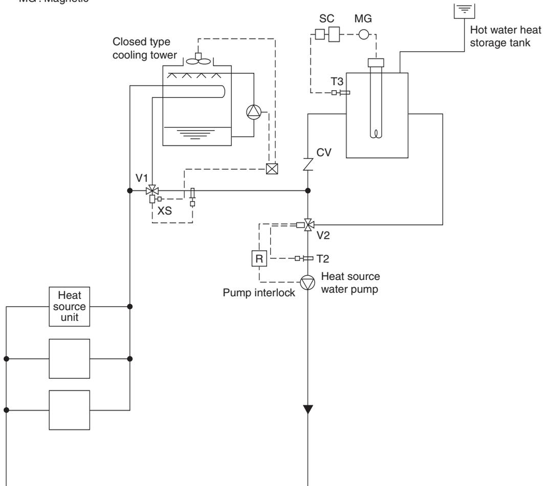
In the summer, as the circulation water temperature rises exceeding the set temperature of T1, the bypass port of V1 will open to lower the circulation water temperature. In the winter, if the circulation water temperature stays below 25°C, V2 will open/close by the command of T2 to keep the circulation water temperature constant.
