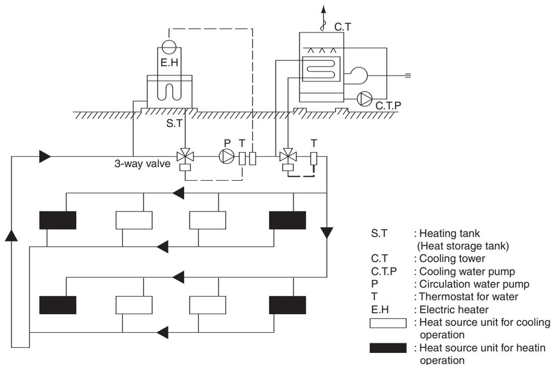
The indoor unit and refrigerant piping system are excluded in this figure.
